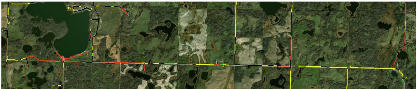
Powerline distribution network coded by vegetation encroachment severity – red (high), yellow (moderate), green (low), black (none).
