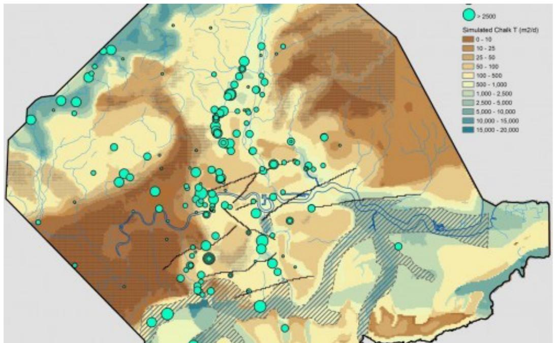
**4** In the confined aquifer there is equivalence between the effects of linear barriers versus low permeability. Model testing, using manual and automated algorithms (such as PEST) was used to investigate aquifer transmissivity within the confined aquifer, with special emphasis on evaluating the role of faults in controlling rates of drawdown and recovery.
