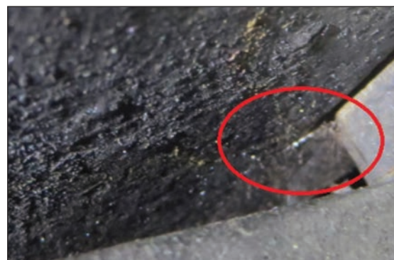
(e) Hair-line crack on a spider arm support ledge.
