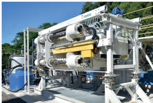
Metso’s pilot VPX filter press unit is installed in Brazil and is ready to perform all tests on an industrial scale, according to Rodrigo Gouveia
