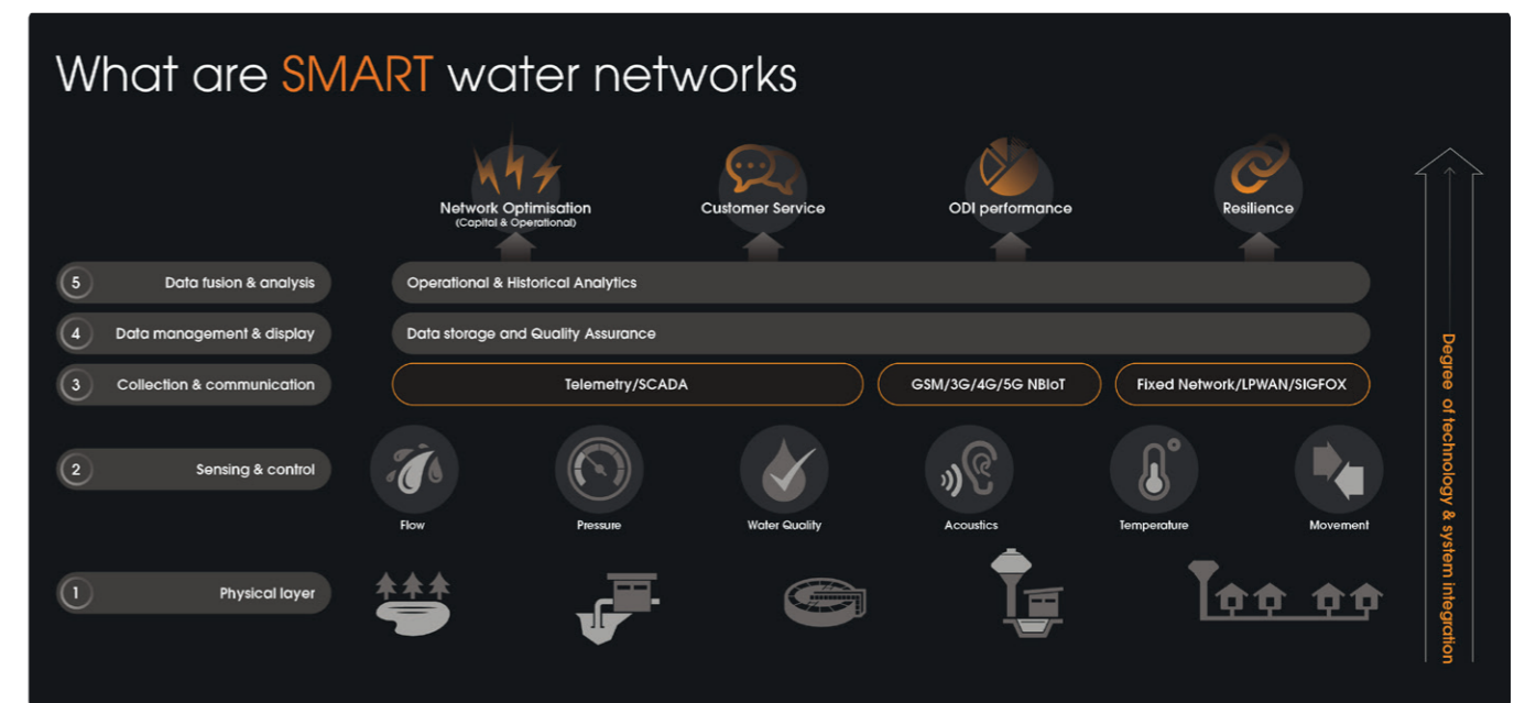
Fig.2 Five layers of smart architecture
