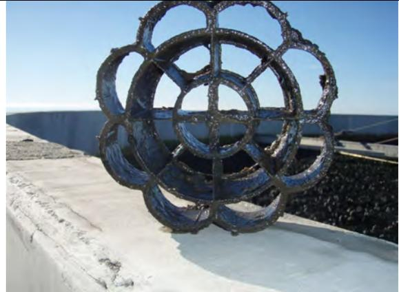
*View of a Plastic Media (Petal) piece showing biomass growth (with 1 – 2mm covering) – taken from the full scale Biological Trickling Filter Plant*
